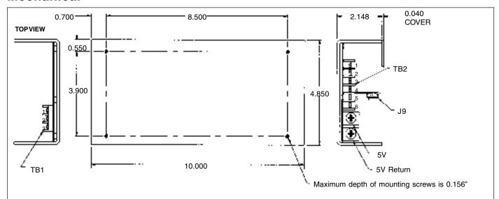
NOTES: All measurements are in inches FAN MOUNTED ON COVER ADDS 1.30".
